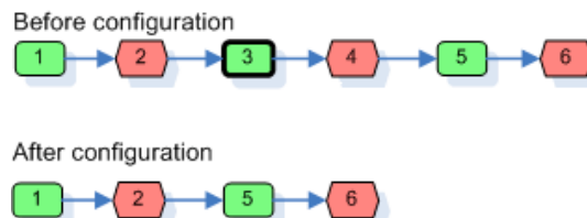
Figure 92: Deletion of configurable function (case enclosed)
